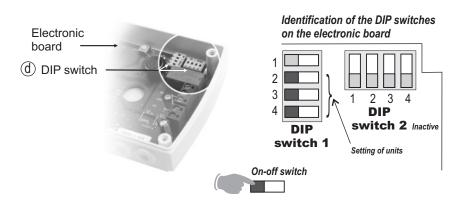
To configure the transmitter, it must not be energized. Then, you can make the settings required, thanks to the DIP switches (as shown on the drawing beside). When the transmitter is configured, you can power it up.
